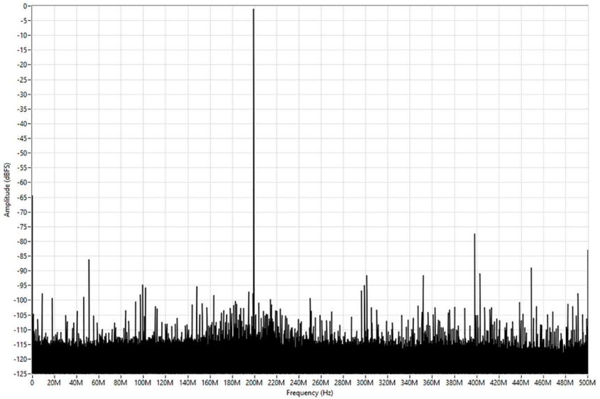
Channel-to-channel crosstalk AC-coupled, measured
