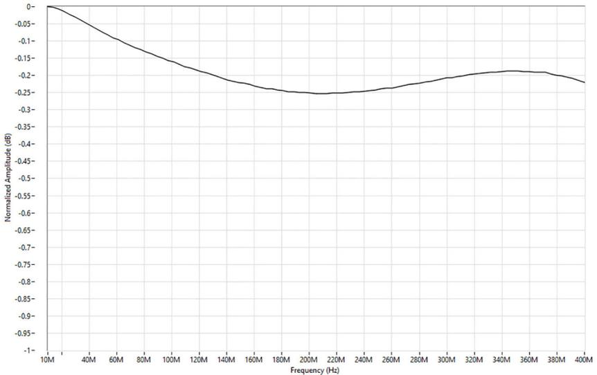
**Figure 9. DC-Coupled Frequency Response, Measured**
