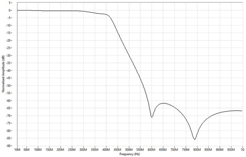
**Figure 10. DC-Coupled Frequency Response Zoomed In, Measured**
