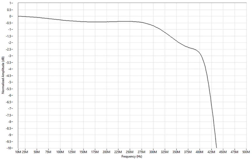
**Figure 11. Input Return Loss, Measured**
